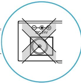
The receiver is powered from the Netvio matrix device over the category cable. A local power supply is not required.
