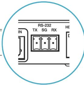
Connect TX to RX, RX to TX and SG to ground when connecting to 3<sup>rd</sup> party devices.
